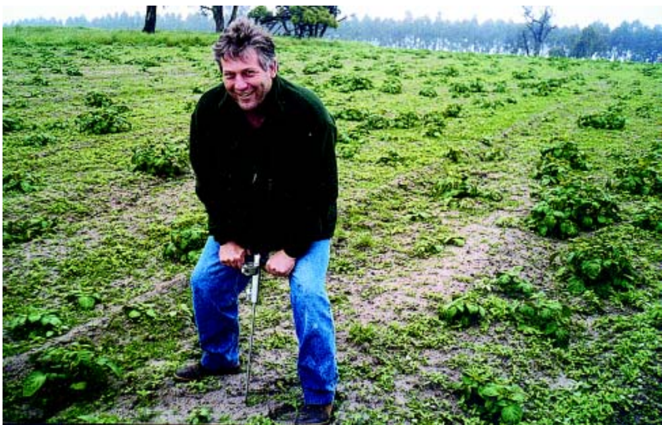
Grower Peter Abel tests the soil compaction in his nicknamed "concrete paddock" with a new agronomic tool called a penetrometer.
